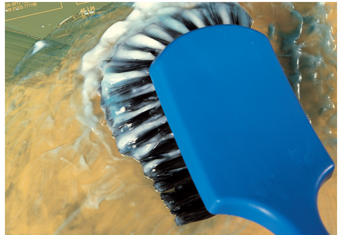
AutoStrip Gel adheres to the screen surface, enabling faster and more efficient stencil removal.
