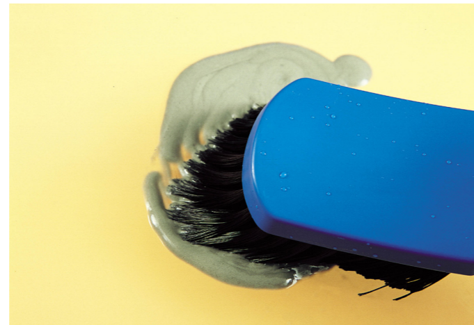
New mesh is abraded with Autotype Autoprep Gel to ensure optimal stencil adhesion, particularly when using stencil films.
