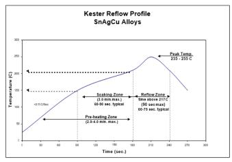
The recommended reflow profile for R520A made with SAC alloys is shown here. This profile is simply a guideline. Since R520A is a highly active solder paste, it can solder effectively over a wide range of profiles. Your optimal profile may be different from the one shown based on your oven, board, and mix of defects. Please contact Kester if you need additional profiling advice.
