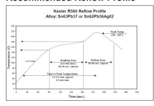
The recommended reflow profile for R560 made with either the Sn63Pb37 or Sn62Pb36Ag02 is shown here. This profile is simply a guideline.
