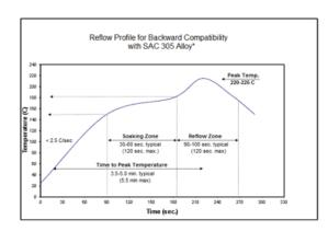
\* This profile is simply a guideline. For a reliable solder joint the reflow profile must produce a homogenous mixing of the tin lead alloy with the lead-free component sphere. The mixing level between the tin lead and lead-free alloy is a function of reflow peak temperature, time above liquidus, component sphere size and sphere alloy. Your optimal reflow profile may be different from the one shown based on your oven, component sphere size and sphere alloy.
