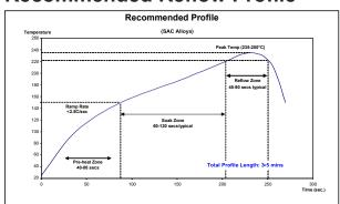
Full convection reflow method is most commonly used to reflow the EM907 formula. The recommended convection reflow profile for EM907 made with either the Sn96.5Ag3.5 or SnAgCu alloys is shown here.
