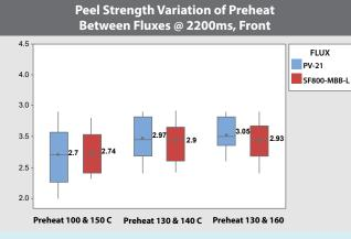
Good soldering and peel strength are seen for all MBB Fluxes.
