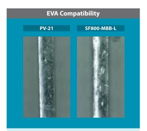
No yellowing and bubbling of EVA in any of the flux coated ribbon.
