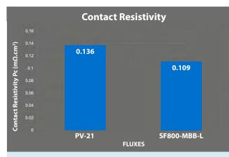
All MBB Fluxes show low contact resistivity, eliminating the risk of high voltage drop in PV module system.
