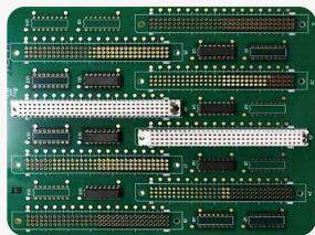
Test Vehicle: Multek PCB PCB Thickness: 2.4mm Alloy: SAC305
