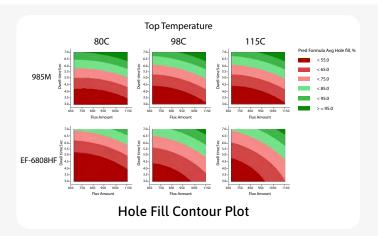
ALPHA EF-6808HF & Kester 985M demonstrate outstanding hole-fill performance across different preheating temperatures.
