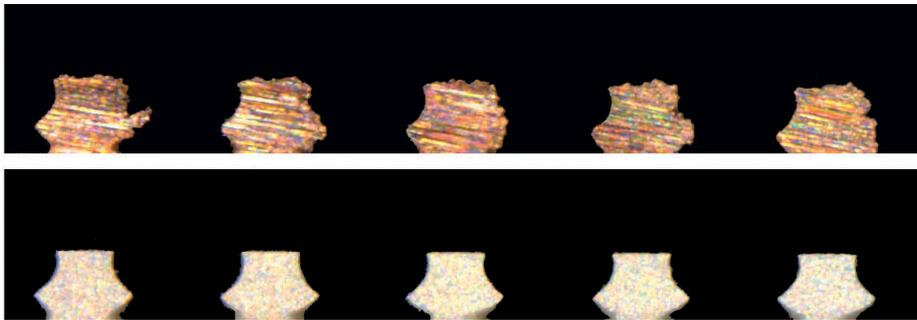
**PackagePrep** prepares and plates the exposed copper alloy edges of QFN packages. The metal coating preserves solderability, meeting JEDEC standards. The soldered coating allows for a three dimensional solder joint that is stronger and more easily inspected than alternative technologies.
