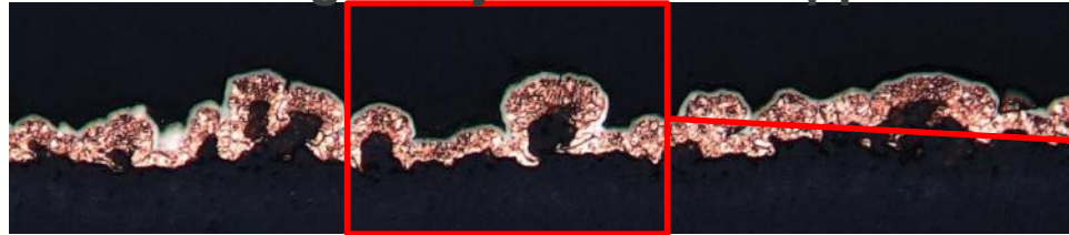
Cu grain structure after peroxide etch.
