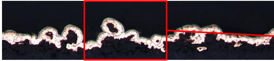
Cu grain structure after peroxide etch.
