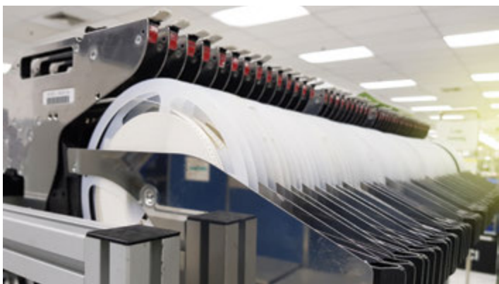
ALPHA Exactalloy Tape and Reel Preforms enable the use of standard pick and place equipment.
