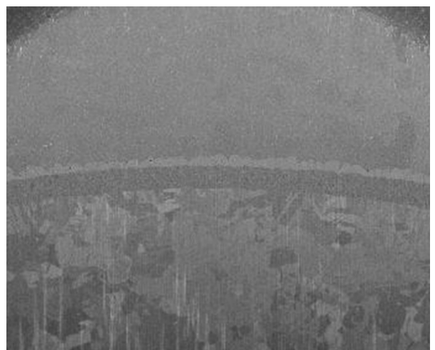
Superior barrier performance after 10x reflow, 1000 hours at 150°C
