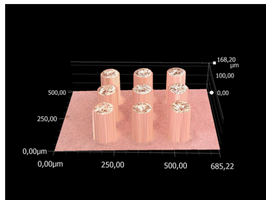
Figure 22. Impression of Pillar Plating works
