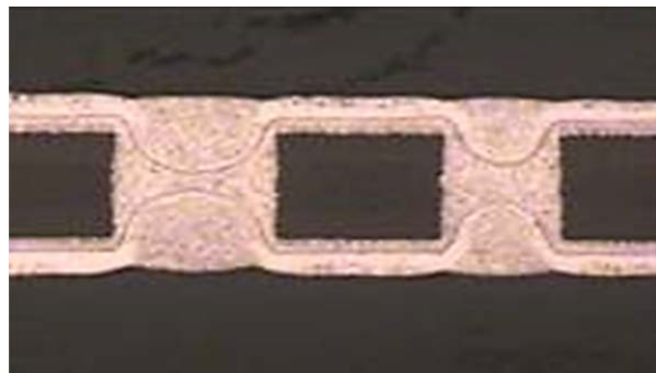
Figure 19. Two-step bridge & fill of TH's
