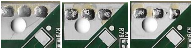
Figure 20a: Solder spread: as plated tin (E) with low SMAP
