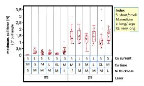
**Figure 3:** Comparison of ns- and ps- laser ablation for plated contact formation (LIP-Ni/Cu + immersion Ag capping) as outlined in Figure 1.
