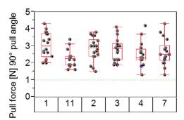
**Figure 4:** Test data from pull testing. Interconnection ribbons soldered to the busbars are pulled off under a  $90^{\circ}$  angle to detach from the solar cell that is kept down.
