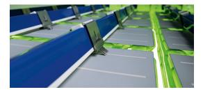
**Figure 6:** RENA has a patented approach to pass the plating current in a controlled way in reverse direction through the pn junction of p-type solar cells. The solar cell rear sides are kept dry while illuminating the immersed front sides on which the contacts are plated..
