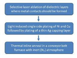
**Figure 1:** Applied simple process flow to form plated contacts with Ni as barrier and interface layer and Cu as main conducting material.
