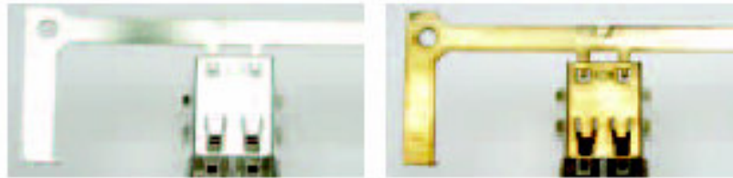
Figure 4. Deposit discoloration after component has been subjected to steam age testing
