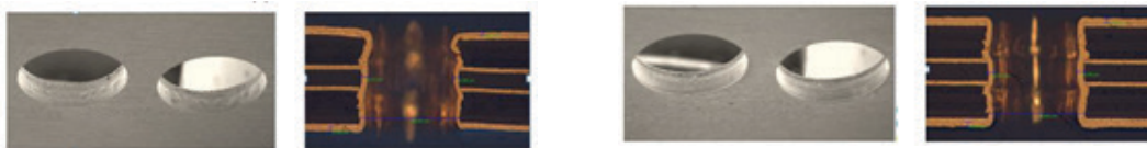
7 Mil Via on AP Material - Left: Conventional Electroless Copper, Right: Via Dep 4550
